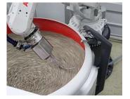
Innovative solutions in automation technology make it possible to use conventional processes such as barrel finishing for new applications in automated single-part processing.
