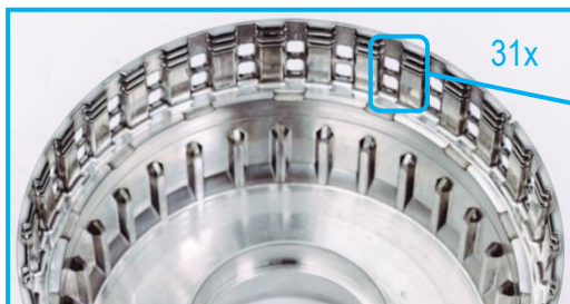
Disk carrier deburring areas
