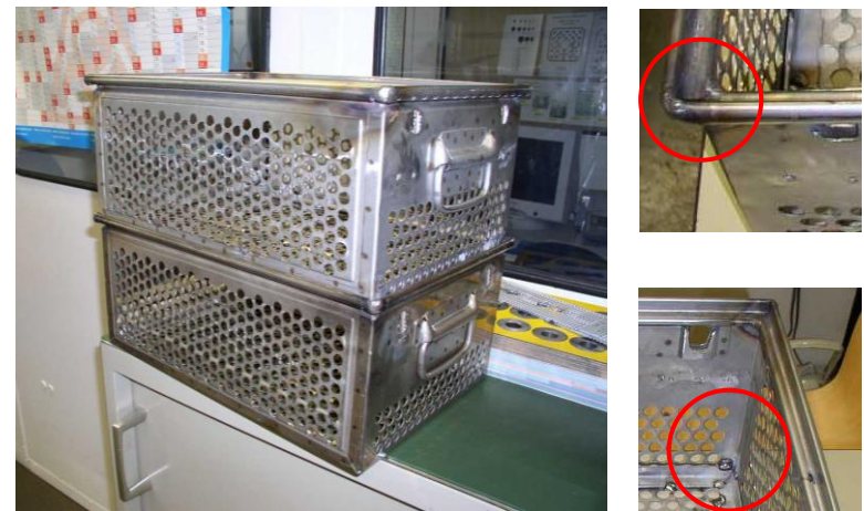
Fig.: Non-Metallform product – compact design, horizontal surfaces at bottom and stacking frame
