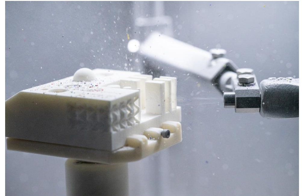
Sample part blasting with plastic blasting medium
