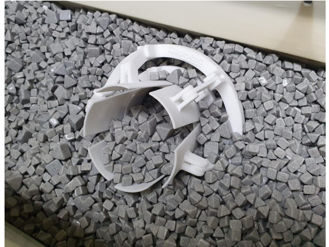
SLS - component in vibratory grinding machine [Source: apc-tec GmbH ]
